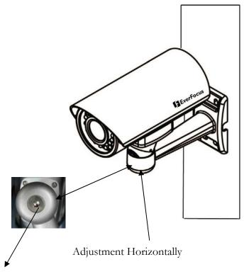
Note: Before you adjust camera's angle, please use Hex key Wrench to loose the screw first. To adjust the angle easier and to avoid paint-off scratches the bracket.
