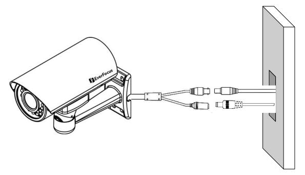
2. Fix the camera to the wall by using the 4 screws.
