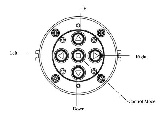
There are two modes in "Control Mode" button. When power is on, it turns to green light. Press "Control Mode" can toggle switch green light and red light.
