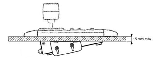
The drawing shows the mounting position of the fixation brackets.
