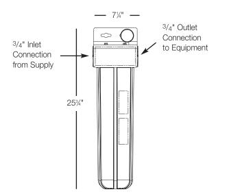
Mounting Depth: 8.5" Operating Weight: 30 lbs. Allow a minimum of 4" clearance under the filter to facilitate cartridge change.
