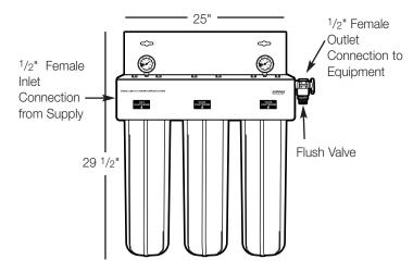
Mounting Depth: 15 <sup>1</sup>/<sub>8</sub>" Operating Weight: 90 lbs. Allow a minimum of 4" clearance under the filter to facilitate cartridge change.
