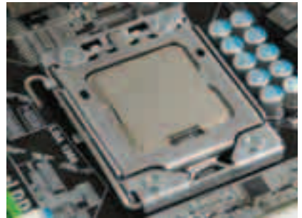
Align notches with notches on the CPU
