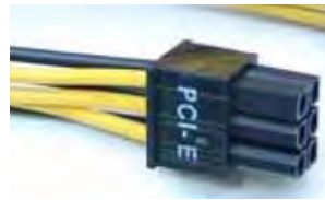
6-pin (3x2) PCI-E connector
