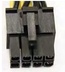
8-pin (4x2) PCI-E Connector
