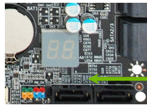
Debug LED with CPU Temperature Monitor
