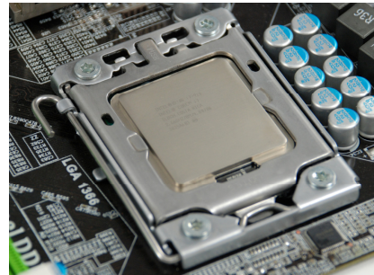
Align notches with notches on the CPU
