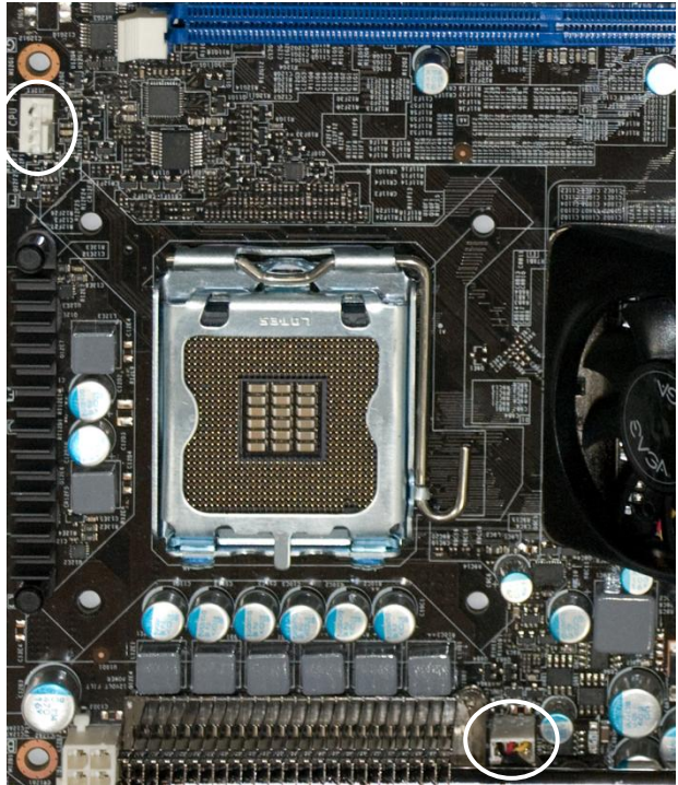
EVGA nForce 780i SLI SPP/MCP fan connector
