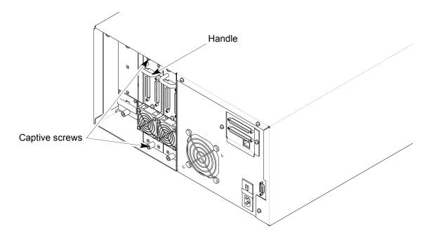
**3.** Remove the drive carrier by grasping the handle and pulling it straight out of the library. The drive carrier weighs about 5 pounds; make sure you support the bottom of the carrier as you remove it.
