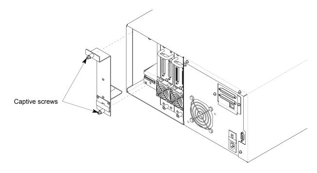
**2**. When the screws are loosened, remove the drive access cover.
