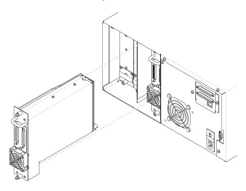
**2**. Tighten the captive screws on each end of the drive carrier to 8.0 inch-pounds (9.2 kg-cm) of torque.
