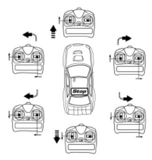
Set the car and transmitter Power Switches to "On." The car is ready for use. Use the transmitter's control levers to steer the car. (See diagrams on next page).
