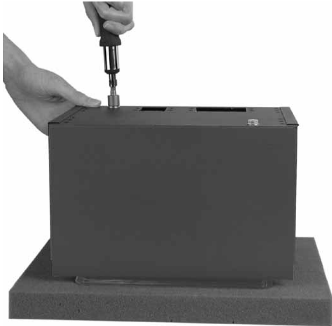
Figure 25. Attaching the Clamshell
