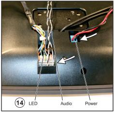
**15.** Replace the orange 2-pole captive screw connector on the provided power supply with the blue connector from the power cable disconnected in step **14**.
