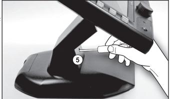
6. At the top, the two plastic plates covering the stand are held together by four locking tabs on the back cover plate fitting into four slots on the front cover plate. Squeeze the sides of the front plate at the top so that the tabs are no longer seated in the slots.
