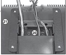
22. Plug in the rear panel cables, as required.
