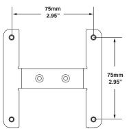
The Extron® VM 700T is an adapter that provides a VESA-mounting option for the TLP 700TV TouchLink<sup>™</sup> panel.
