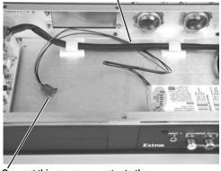
Connect this power connector to the interface's power connector
