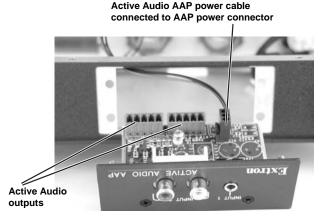
The Active Audio AAP plate's power and audio connections must be wired before mounting the AAP plate in the interface. Both the provided Active Audio AAP power cable and the included captive screw audio connectors are keyed to prevent incorrect connections.
