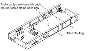
Connect powered speakers or another audio device to the included captive screw connectors. Insert the audio device wires into the captive screw connector and tighten the captive screws to fasten the wires, then insert the wired audio connector into the audio output connector of the Active Audio AAP plate before installing the AAP plate into the interface.
