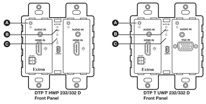
Figure 14. Transmitter LED Indicators
