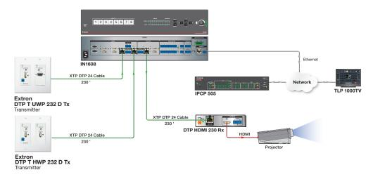
Figure 1. A Typical Transmitter and Receiver Application
