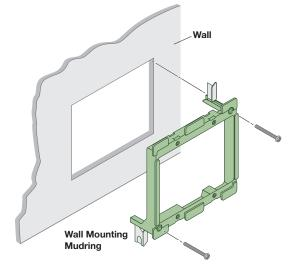
Figure 3. Installing the Mud Ring
