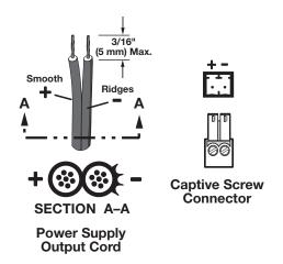
Figure 10. Power Connector Wiring
