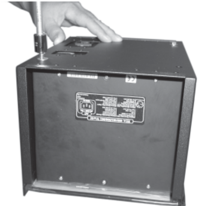
Figure B-3 — Attaching the clamshell
