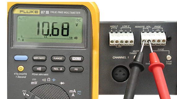
Measuring control voltage for a Peavey UMA™ 35T II: meter leads are oriented correctly
