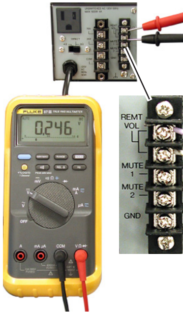
Measuring control voltage for a TOA A-903MK2 amp
