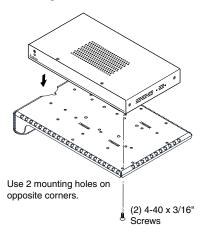
Secure the device to the plate with 4-40 screws.
