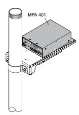
Attach input and output cables to the mounted device and thread them through the access hole in the projector pipe to the inputs and the display device. Use the remaining tie wraps for cable tidying.
