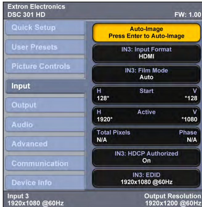
Figure 7. OSD Menu – Input Submenu
