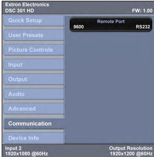
Figure 13. OSD Menu – Communication Submenu
