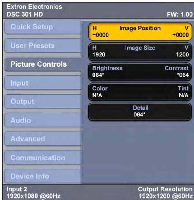
Figure 6. OSD Menu – Picture Controls Submenu
