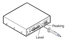
Level adjustment control — The Video Output Level control alters the brightness of the displayed image. To adjust the video output level, view the display while using a small, flat-blade screwdriver to rotate this potentiometer.
