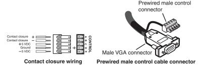
**NOTE** The contact closure pins on the RGB 580xi's front panel are not to be used for horizontal shift control. See the horizontal shift control wiring in the 15-pin HD pinout table in **Step 3**.
