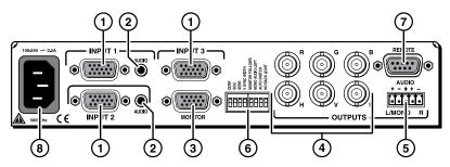
**Step 3: Connect Video Inputs** — Connect an RGBHV, RGBS, RGsB, or RsGsBs video input to each 15-pin HD connector (①), as desired.
