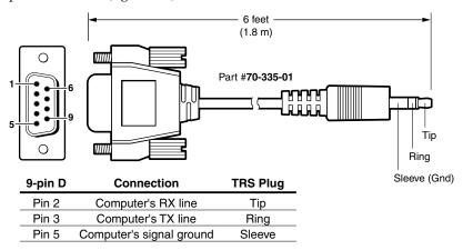
Figure 2-7 — Optional 9-pin TRS RS-232 cable
