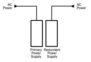
Figure 1-2 — Redundant power supply backs up primary
