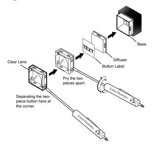
Figure 7-4 — Illuminated button label replacement
