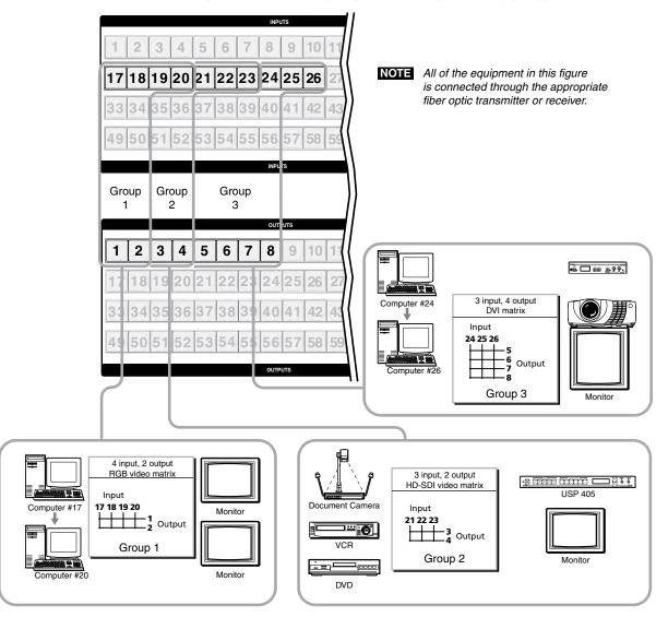
Figure 3-4 — I/O grouping of incompatible video formats
