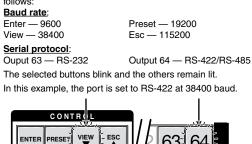
4. Exit *Serial Port Selection and Configuration* mode: Press and release an output button.
