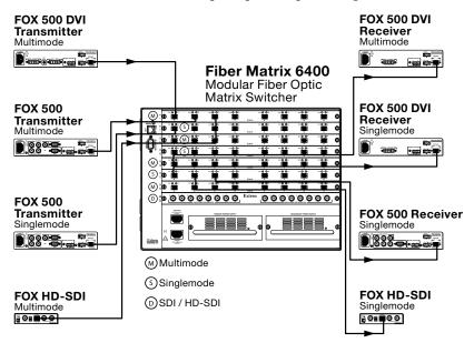
Figure 1-1 — Typical Fiber Matrix 6400 application
