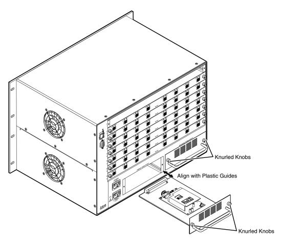
Figure 7-3 — Power supply replacement
