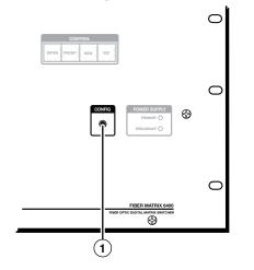
Figure 2-6 — Front panel configuration port
