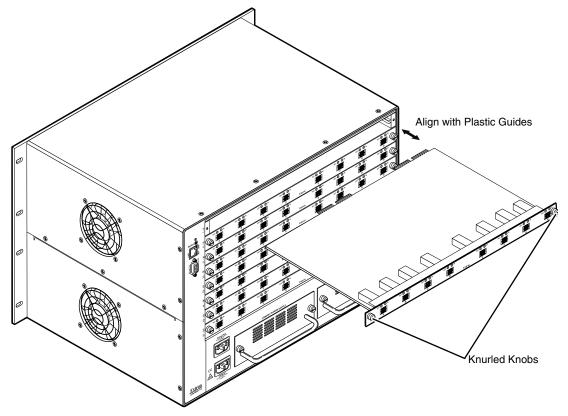
Figure 7-2 — I/O board replacement
