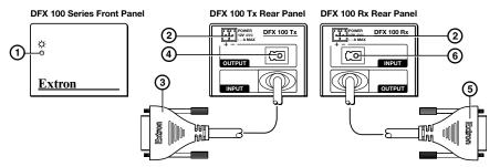
1. Connect one of the provided 12 VDC power supplies to the rear panel captive screw connectors of the transimtter and the other to the receiver ((2)).
