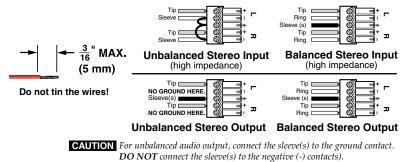
Audio Output connector — Connect a balanced or unbalanced stereo or mono audio device to this 3.5 mm, 5-pole captive screw connector. Wire the connectors as shown above.
