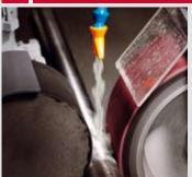
Add-on module for finishing and polishing applications on round, ferrous and non-ferrous stock – from rough grinding to mirror polish.
