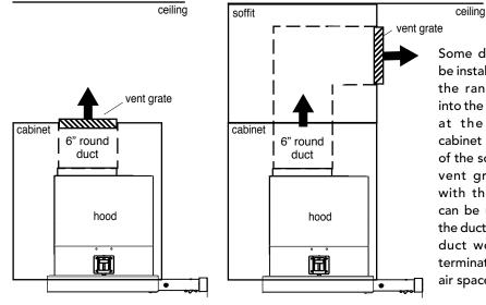
Some ductwork must be installed to exhaust the rangehood back into the kitchen, either at the top of the cabinet or at the face of the soffit. A plastic vent grate supplied with the rangehood can be used to cover the duct opening. This duct work must not terminate into a dead air space.
