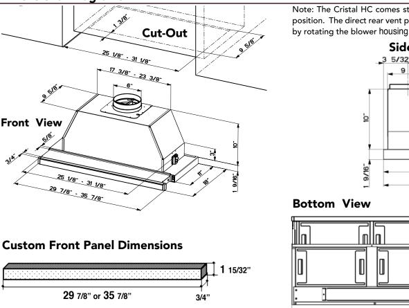
Note: The Cristal HC comes standard in the top vent position. The direct rear vent position can be achieved by rotating the blower housing.
