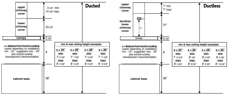
The ducted Axia Isola chimney can be adjusted for ceilings between 7' 5 5/ 8" and 8' 10 5/ 8" depending on the distance between the bottom of the hood and the cooktop (distance x in above DUCTED diagram). The ductless Axia Isola chimney can be adjusted for ceilings between 7' 10 5/ 8" and 8' 10 5/ 8" depending on the distance between the bottom of the hood and the cooktop (distance x in above DUCTLESS diagram).
