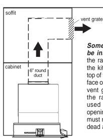
Some ductwork must be installed to exhaust the rangehood back into the kitchen, either at the top of the cabinet or at the face of the soffit. A plastic vent grate supplied with the rangehood can be used to cover the duct opening. This duct work must not terminate into a dead air space.
