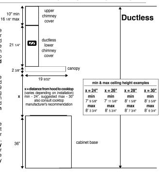
Note: If 24" or 30" High Backsplash is being installed, the distance between the bottom of the hood and the cooktop (distance x in diagram) is equal to the height of the Backsplash.
