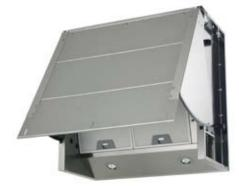
The Jewel comes with an unfinished metal front which you can attach to your custom cabinet face. This 18" tall rangehood replaces your upper cabinet, and when tilted out, extends 9.5", for a total depth of 20.5" from front to back, providing adequate coverage for most cooktops.
