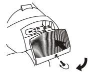
Reattach the lens and fasten the screws.
