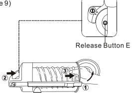
3 Clean the main filter and prefilter with a soft-bristled brush and rinse with cold water. Allow both items to dry completely.
