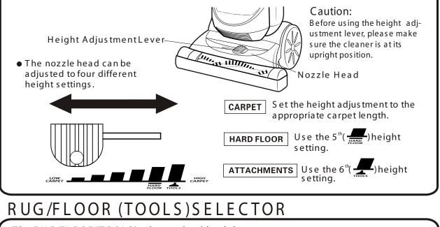
The RUG/FLOOR (TOOLS) selector should only be adjusted while the vacuum cleaner is turned on and in the upright position.
