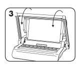
3. Test punch scrap sheets to check edge guide setting.
