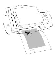
The finished sheet will emerge from the sheet exit (F) by itself. Remove it from the open cover only after it has completely cleared the exit.
