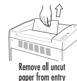
Press Forward for 5 seconds to clear cutters. Press Forward button again to resume Auto start
