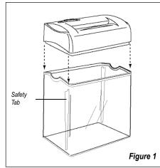
NOTE: This shredder will operate only when used with the supplied basket. The supplied basket has a built-in safety feature which prevents the shredder from operating if used with any other basket or if improperly assembled.
