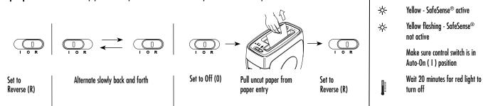
ATTENTION: If the SafeSense® light remains on, you must engage the So Override Switch in order to perform steps above. Once the jam is cleared, reset the SafeSense® feature. (See SafeSense® instructions below.)
