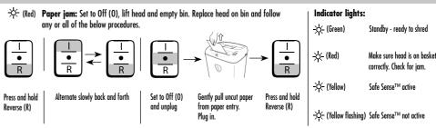
Note: If Safe Sense™ light remains on, you must engage override switch in order to perform above steps.
