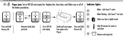
Note: If Safe Sense™ light remains on, you must engage override switch in order to perform above steps.
