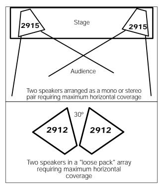
If the speaker is part of a tightly packed array (see figure below), the coverage pattern should be modified to reduce overlapping radiating patterns of multiple drivers. (See the section on "Horn Inserts" for more information.)
