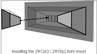
Reinstall the grille by placing one side of the grille under the side cleat, then gripping the grille on the top and bottom, bend the other end under the cleat at the opposite end of the cabinet. With the inserts installed, the horizontal coverage angle is reduced to 60°.
