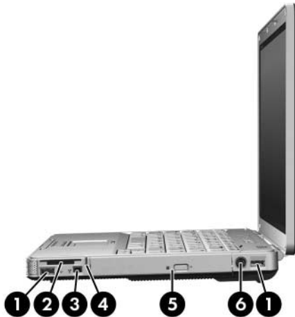
Right-Side Components, HP Compaq nx4820 and Compaq Presario V2400
