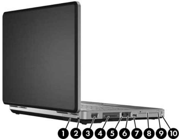
Rear and Left-Side Components, HP Compaq nx4820 and Compaq Presario V2400
