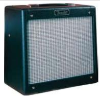
The 15-watt, single-channel Pro Junior is a small all-tube amp, pure and uncomplicated. Features include a single 10" Eminence® speaker, two EL-84 output tubes, two 12AX7 preamp tubes, Volume and Tone controls, black textured vinyl covering and silver grille cloth.
