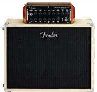
High-quality companion stereo enclosure for the Acoustasonic<sup>™</sup> Ultralight amp. Features include Italian poplar plywood construction, internal cabinet divider panel, two 8" Eminence<sup>®</sup> low-frequency speakers and two high-fidelity 1" dome tweeters, and magnetic docking system for secure attachment of amp to enclosure. Rated at 2x125 watts (stereo) at 4 ohms per side.
