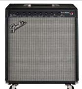
The 140-watt Jazz-King is a solid-state amp based on our successful Steel King, with a lighter speaker and a flatter preamp voicing specially tailored to jazz guitar. Features include a single 15" Eminence® speaker, a versatile preamp, XLR output, effects loop, tuner output with mute, limiter, and spring Reverb. Three-button footswitch (for Tuner Mute, FX loop, and Reverb) and fitted cover included.
