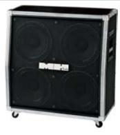
Slant-baffle companion enclosure for the MH-500 Metalhead, with four heavy-duty 100-watt Celestion® G-12K100 speakers and matching "flight case" hardware. Features include premium birch construction, pop-out casters, perforated metal grille and angled nickel-plated steel edge reinforcement. Handles 400 watts RMS (4 ohms total impedance).
