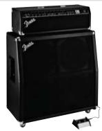
The FM 412SL is the slant-enclosure companion to the FM 100H head, and easily handles 100 watts of power. It contains four 12" heavy-duty Fender® Special Design speakers. Details include premium wood-ply construction (not particle board!), pop-out swivel casters, chrome hardware and black vinyl covering and grille cloth. 4 ohm impedance.
