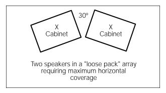
NOTE: When setting up your X Series enclosures, be sure to place the cabinets in such a way as to minimize overlapping radiating patterns.
