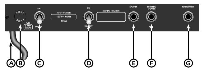
**A. LINE CORD** - The Vibro-King is equipped with a grounding type supply cord to reduce the possibility of shock hazard. Be sure to connect it to a grounded AC receptacle. **DO NOT ALTER THE AC PLUG.**
