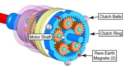
Another feature of the C12 gearbox is the integral shaft-lock to assist in bit changing. The motor can rotate the drill chuck, but the drill chuck cannot
