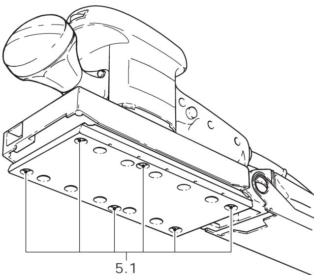
The standard STF 115 x 225 mm Stickfix sanding pad can be exchanged for the 115 x 225 mm sanding pad for use with clamping paper. Loosen the six fastening screws (5.1).
