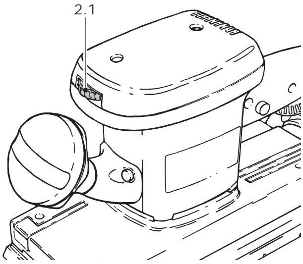
The RS 2 E has an electronic control with which the rotational speed can be varied step-free. This allows the sanding speed to be adapted to the optimum level according to the material concerned.
