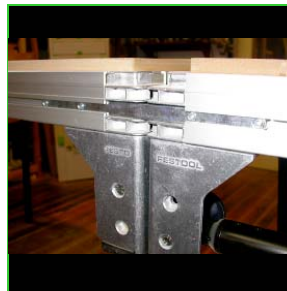
The MFT connectors fit the "T" slots around the perimeter of the MFT
