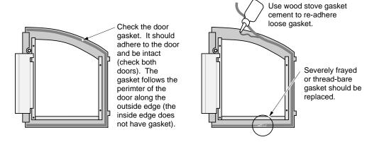
When closing the doors, the handle should pull the doors in and dreate a snug fit. If it
