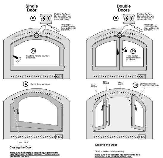
**Warning**: When closing the doors, make sure the door latch does not strike the front of the left side door. This will damage the finish on the doors.
