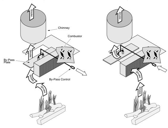
• An optional combustor temperature probe is available from your dealer. It allows you to monitor the combustor temperature, which light off if the temperature is above 600° F.
