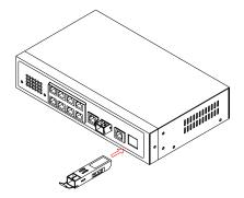
Fig. 2-1 Installation of Optional SFP Fiber Transceiver
