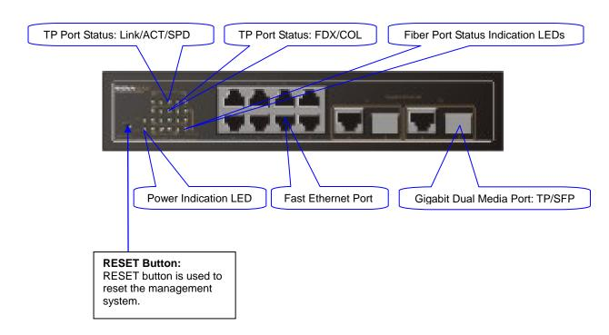
Fig. 1-2 Front View of 8 Fast Ethernet + 2 Gigabit L2 Managed Switch with SFP Module
