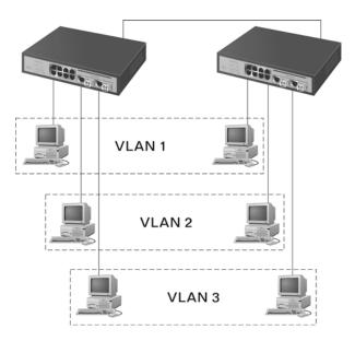
Fig. 2-6 Attribute-based VLAN Diagram
