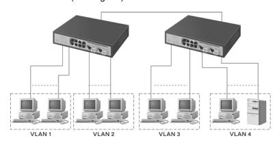
Fig. 2-5 Port-based VLAN Diagram
