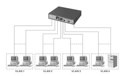
Fig. 2-4 Port-based VLAN Diagram
