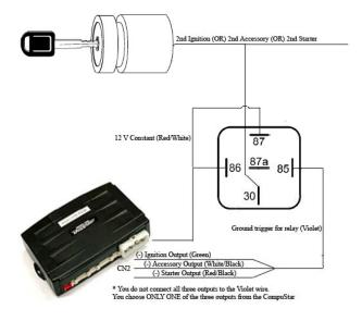
the negative (-) Ignition output from Connector 3, to the short violet wire coming off of the relay, will provide an additional (+) 12V Ignition output from the long blue wire.
