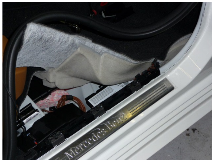
CAN connector, E, C, GLK class under plastic passenger front door
