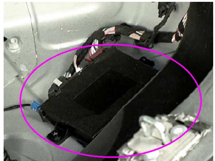
R KeylessGo module -- under cargo area floor
